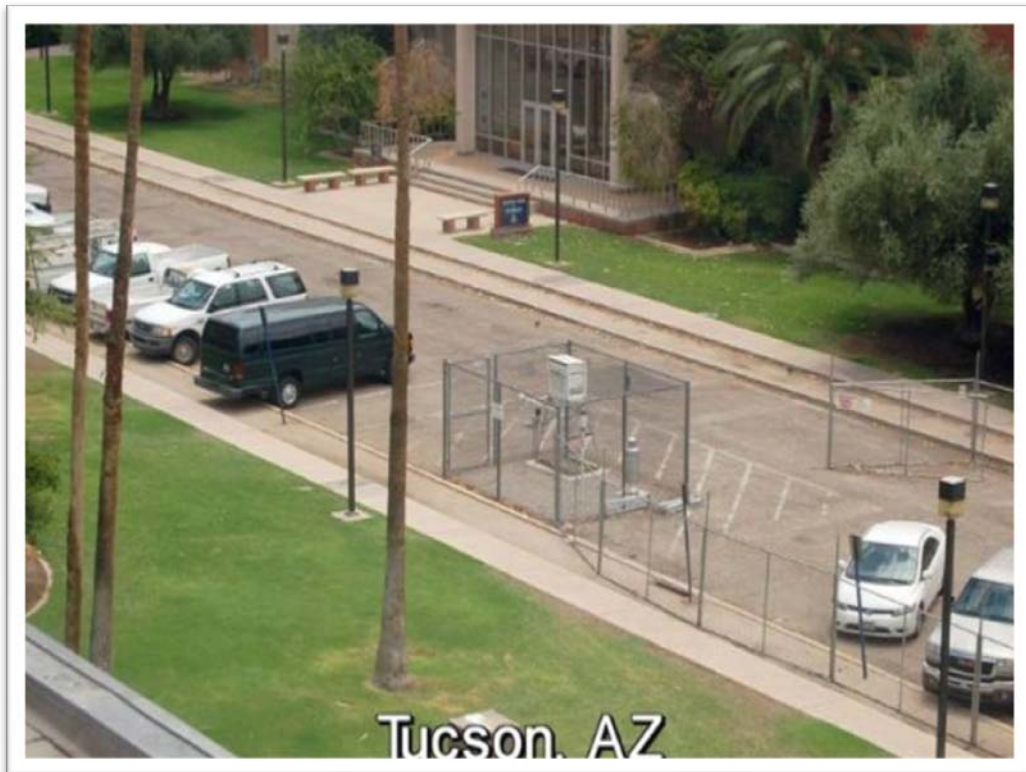
A station at Tucson, AZ, in a parking lot on pavement. (Photo by Warren Meyer, courtesy of surfacestations.org .)
